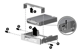
removing a diskette drive from the drive adapter on the 8000 series
